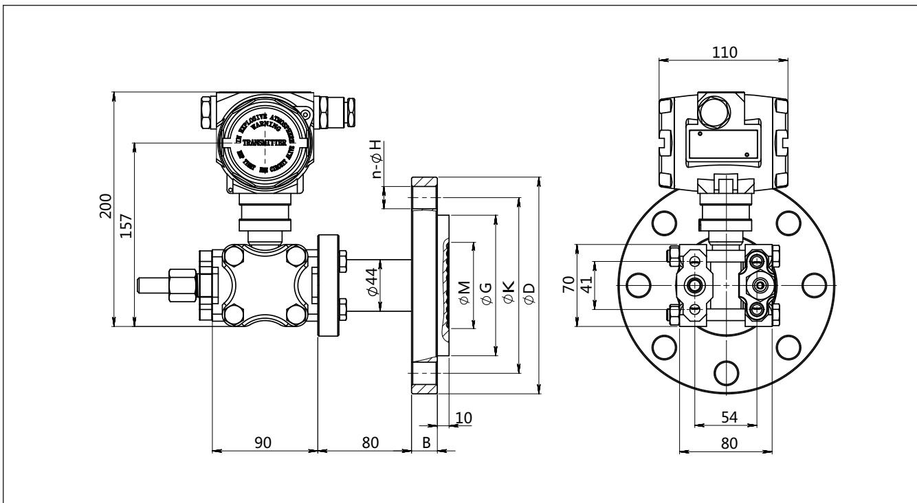
Dual extented diaphragm drawing and dimension without display(A) ( unit: mm)
