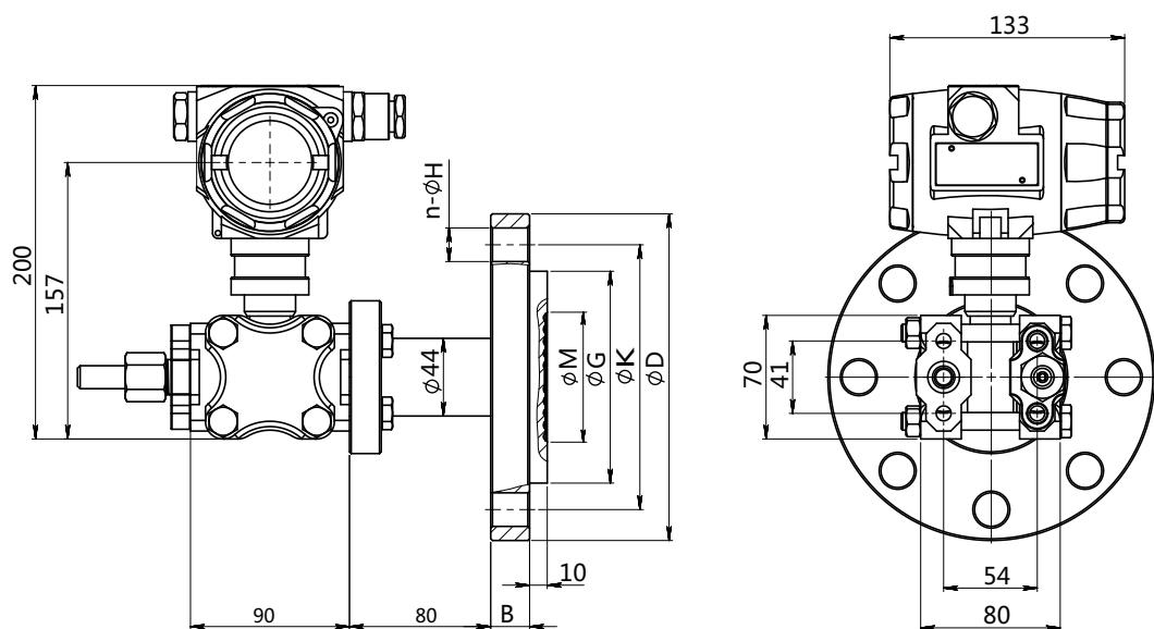
Dual extented diaphragm drawing and dimension with display(C) ( unit: mm)
