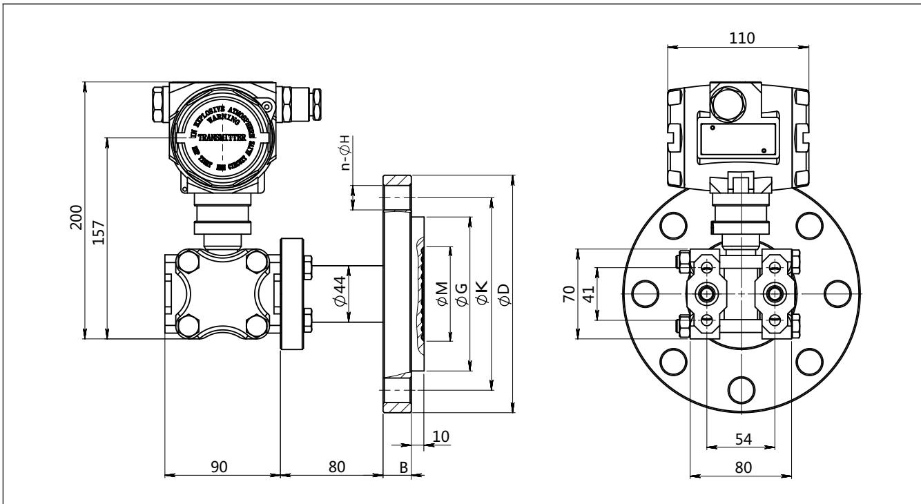
Standard extended diaphragm without display(A) (unit:mm)
